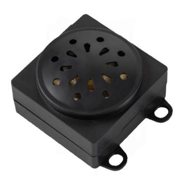
WA-290B- new national standard is a GPS positioning control for e-bike control. It has GSM network remote control, 433M remote controller,GPS real-time positioning, Bluetooth communication, vibration detection, anti-theft alarm and other functions. Through GSM and Bluetooth, the GPS terminal can interact with the background and mobile APP to control the e-bike and upload the real-time status of the e-bike to the server.
