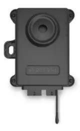
WD-280 is a 4G smart device for the e-bikes with GPS positioning function, it supports UART and Bluetooth communication. Through it, the users can control their e-bike by 4G LTE-CAT1 or 433M remote controller. Besides, the device support GPS real time positioning, vibration detection, anti-theft alarm and so on. Through LTE and Bluetooth, WD-280 interacts with the platform and APP to control the e-bike, and upload the real-time status of the e-bike to the server.
