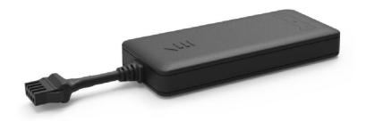
WD-108-4G is a 4G GLONASS/GPS combined tracking device with ACC detection for scooter and car & motor.
