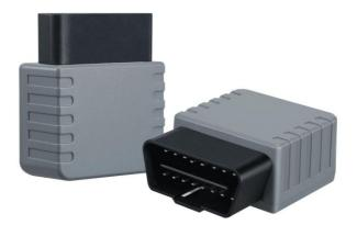
OBD tracker has integrate variety of modules, such as GSM/GPRS module, high-precision GPS module and high-performance three-axis gravity sensor, which can detect the current state and position information of the vehicle in the first time, and send it back to the cloud data platform through the wireless communication network for intelligence analyze and judge.
