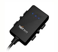
NB-100 is a NB-IOT tracker which supports a variety of satellite navigation systems, including GPS\Beidou\GLANESS\GALILEO and satellite augmentation system SBAS. Besides, it supports NB-IOT networks, and has a built-in antenna design for easy installation. The equipment has built-in backup battery, external power detection, etc., which can realize power failure alarm. Users can check the real-time location and driving trajectory of the vehicle anytime and anywhere online or use the mobile APP.
